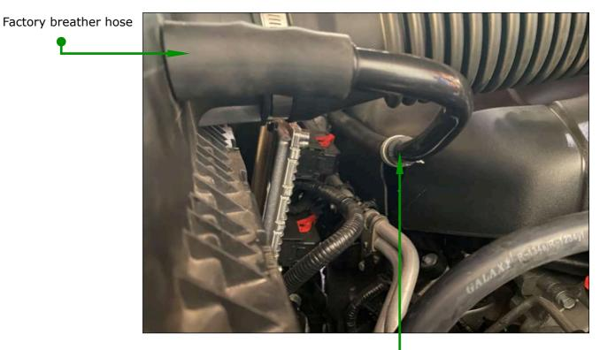
Cut factory breather hose in this location and connect (**OUT**) hose from tank
