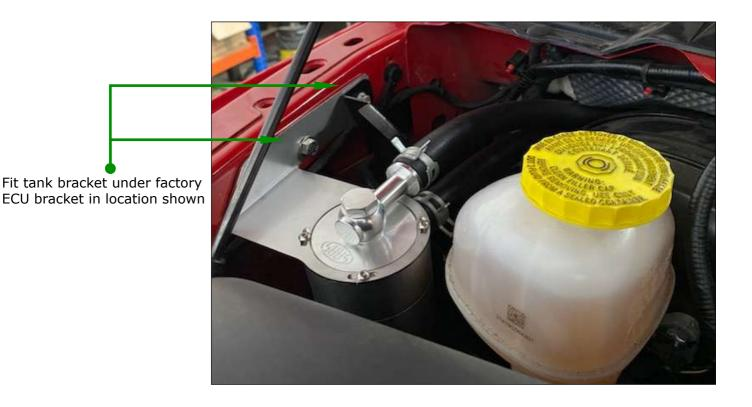
**Step 3:** Locate the factory breather hose shown below and cut the hose on a straight section below the air box to connect the 19mm hose from tank.(See page 4 for layout)
