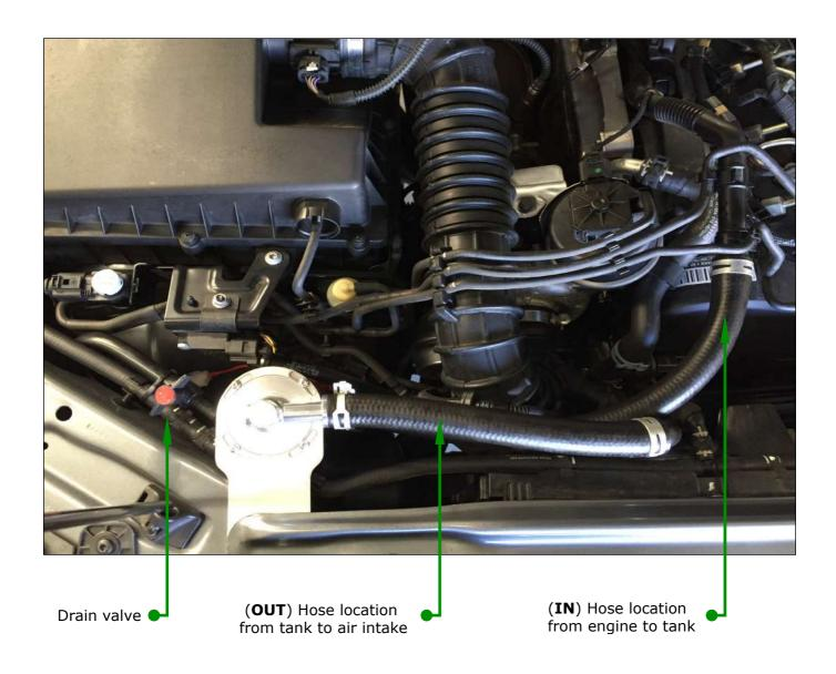
**Step 6:** Cable tie the drain valve in a easy to get to location.(Optional)
