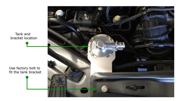
**Step 3:** Locate the factory breather hose shown below and cut the hose on a straight section.
