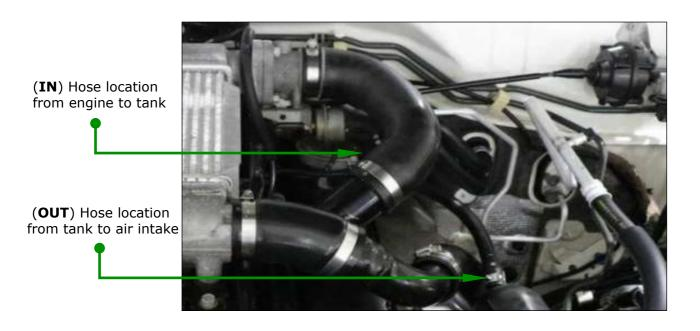
**NOTE:** SAAS recommends checking your catch tank after traveling 1000km to see how much oil has accumulated in the tank. It is important that the build-up of oil does not rise above the internal baffle through to the bronze filter.
