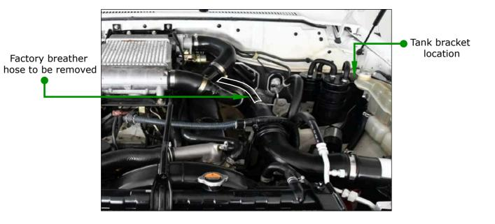
Step 5: Connect (IN) hose from engine to tank in location shown below. (See page 3 for layout) **Step 6:** Connect (**OUT**) hose from tank to air intake in location shown below. (See page 3 for layout) **Step 7:** Cable tie the drain valve in a easy to get to location.(Optional)
