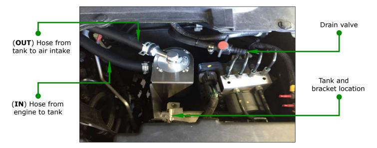
**Step 8:** Cable tie the drain valve in a easy to get to location. (Optional)
