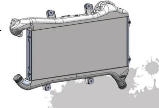
It is then over to our dedicated manufacturing team to manufacture the entire assembly from scratch, this includes the core which is stacked and furnace brazed right here in our Australian head quarters. The whole assembly is then hand TIG welded in a jig to ensure that every intercooler is built to the exact same specification for worry free fitment.
