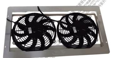
The issue with the OEM top mount intercooler on the 200 Series is that it purely relies on the limited air flow that is fed through to the core from the restrictive factory under bonnet ducting, this seriously compromises the efficiency of the intercooler particularly at lower speeds. The main problem we found during real world testing was that without the PWR Performance Thermo Fan Package the OEM intercooler suffered from heat soak which seriously compromised performance.
